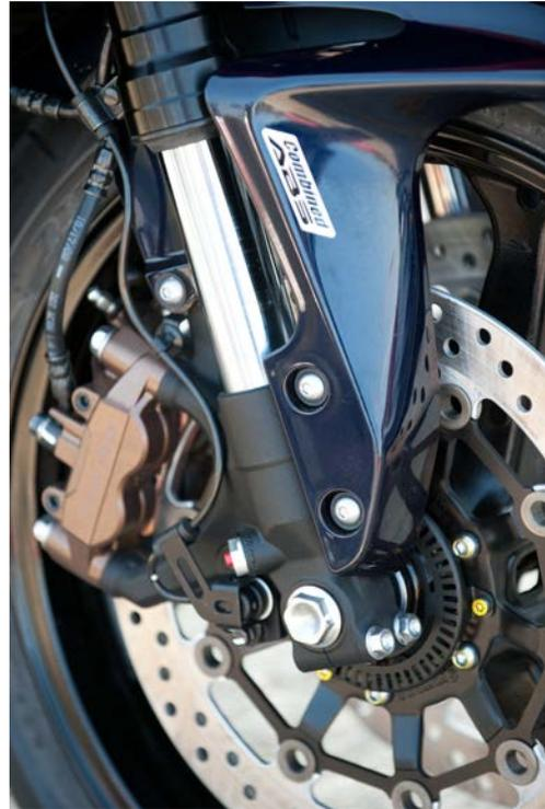
*Front wheel disk brake fitted with ABS*
